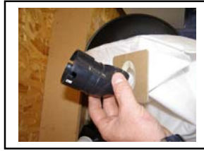
This part of the intake it bayonet mount and can be removed by twisting it anticlockwise and pulling it off. Insert into the new bag and reattach by aligning the two small arrows.
