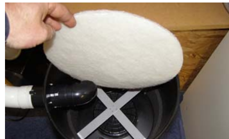
Remove the white nylon mesh filter and tap it against an outside wall to release any dirt. Remove the metal frame below to get access to next filter.
