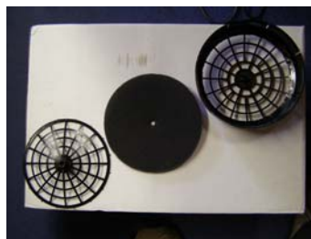
Remove the white nylon mesh filter and tap it against an outside wall to release any dirt. Remove the metal frame below to get access to next filter.
