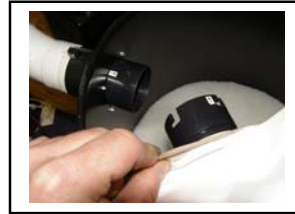
This part of the intake it bayonet mount and can be removed by twisting it anticlockwise and pulling it off. Insert into the new bag and reattach by aligning the two small arrows.
