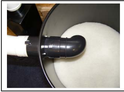
Two piece intake without dirt bag attached Note the two arrows lined-up
